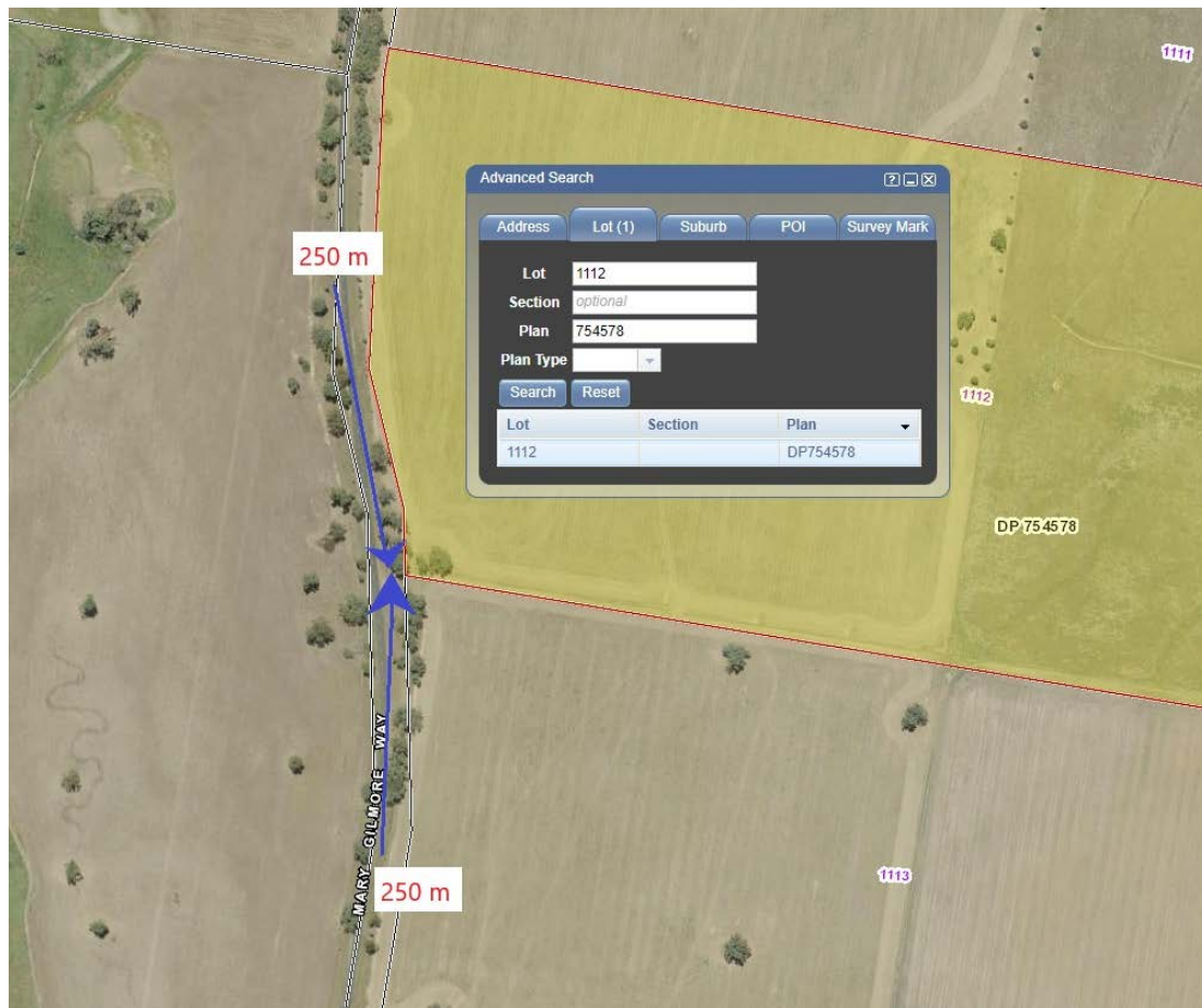
Figure 10. Location plan showing required Safe Intersection Site Distance.
